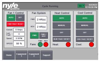
**Fan 1 Control:** allows you to control the fan settings.
