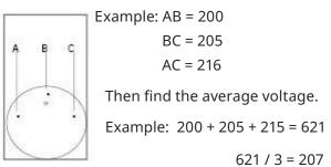
Find the difference between the average voltage and the measured voltages for AB, BC, and AC. This is called the standard deviation. The highest number is your maximum deviation.
