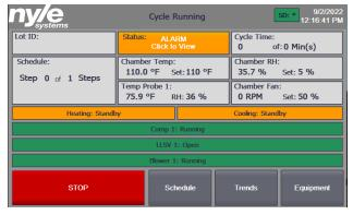
Chamber temperature and relative humidity will be displayed, along with current user set points for desired chamber temperature and relative humidity.
