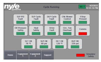
The alarm screen allows the user to view currently active alarm conditions and which equipment have faults.
