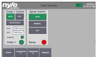
**Comp 1 Control:** allows you to control the compressor as well as monitor the line pressures.
