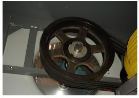
The belt tension must be correct. If too tight, reduced bearing and belt life will result. If too loose, belt life will be shortened due to slippage. The ideal situation would be for the belts to be as loose as possible without squealing.
