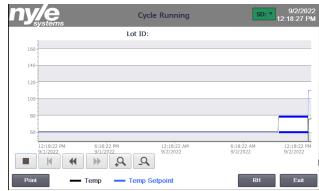
The trend screen lets the user view the previous 24 hours of dryer operation in a graphical display. The system offers two trend screens, one that records system temperature and one that records RH.
